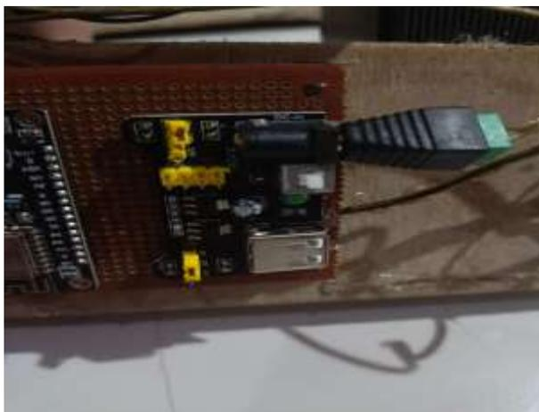
**Gambar 5.** Bread Board Power Supply
